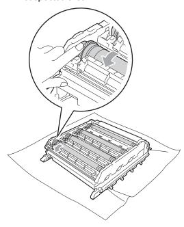
When you have found the mark on the drum that matches the drum dot check sheet, wipe the surface of the drum gently with a cotton swab until the dust or paper powder on the surface comes off.
